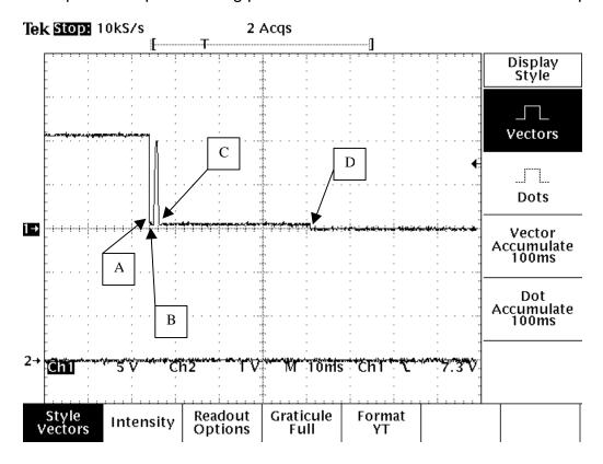
Position A: mechanical switch on VMC is pulling pin 3 low (i.e. door switch)
