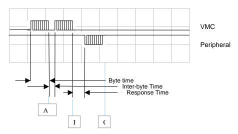
Please note, that the receiving device at the bus (master or slave) will get a receive interrupt (using standard UART devices) only after the byte is fully transmitted. These are the positions A, B, and C in the above diagram.
