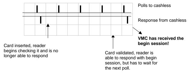
As shown in the above diagram, the time from card insertion to credit being displayed on the vending machine is not specifically related to the polling rate. After the card is inserted, the card reader validates the card. During this time, some card readers are no longer able to answer the poll, others answer with an ACK only.
